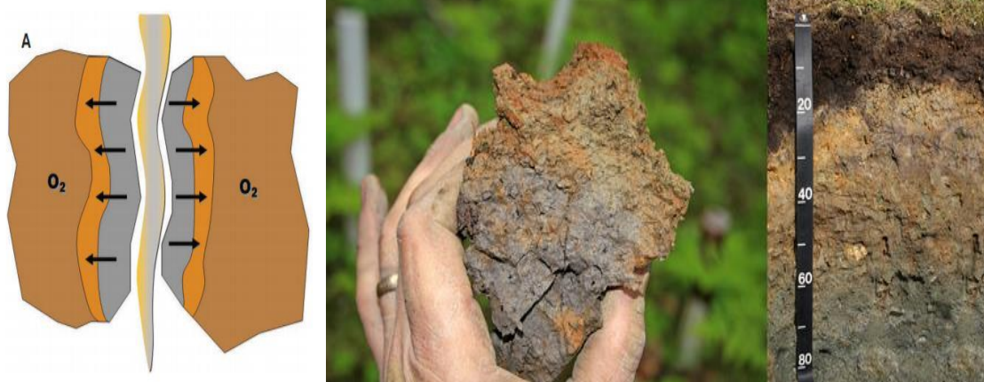
Figure 4.3: The typical formation of a redoximorphic feature within the soil profile (adapted from Jackson et al, 2014)
